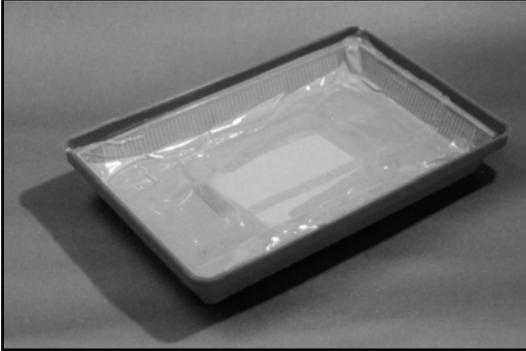
**Figure 2:** Incubator lid taped-up to restrict moisture loss.
